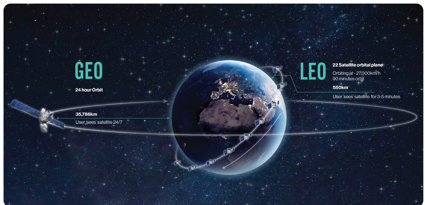
Figure 1: Comparison of Architectures of GEO vs LEO 1 Constellations
